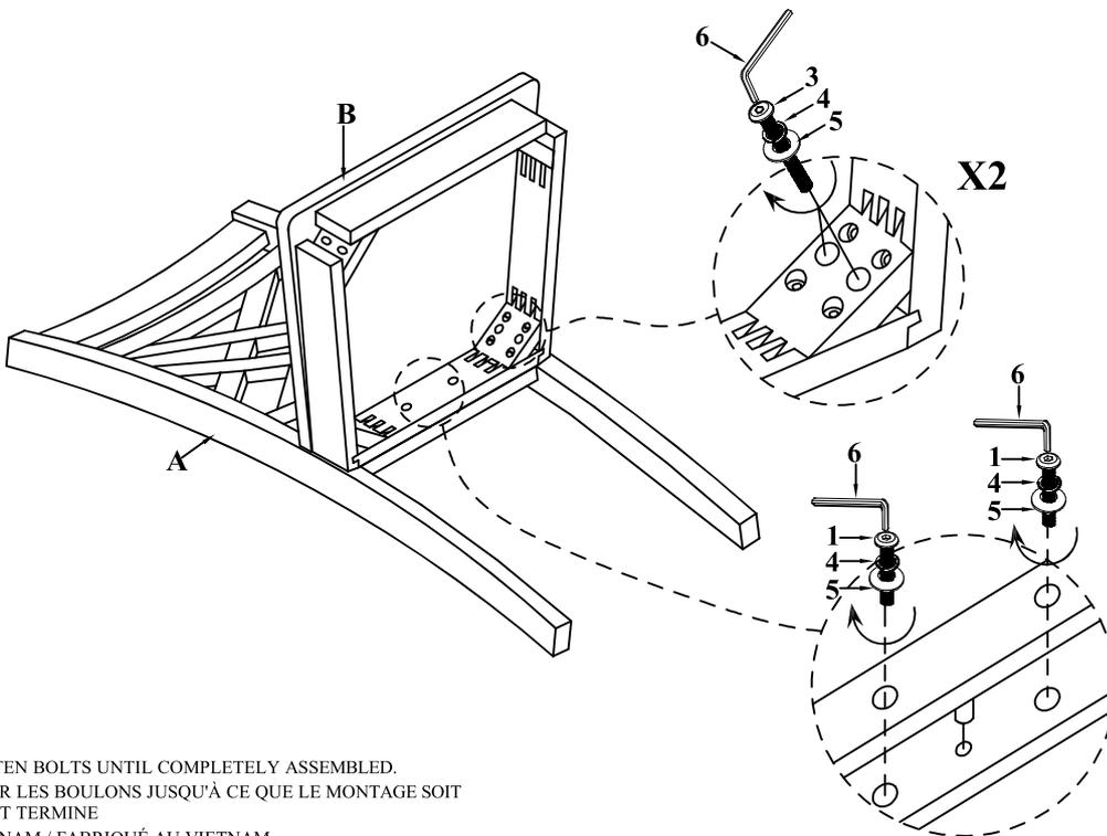
DO NOT TIGHTEN BOLTS UNTIL COMPLETELY ASSEMBLED.
