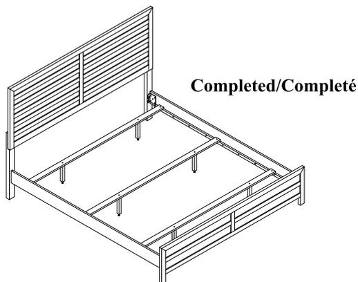
**\*\*DO NOT TIGHTEN BOLTS UNTIL COMPLETELY ASSEMBLED
