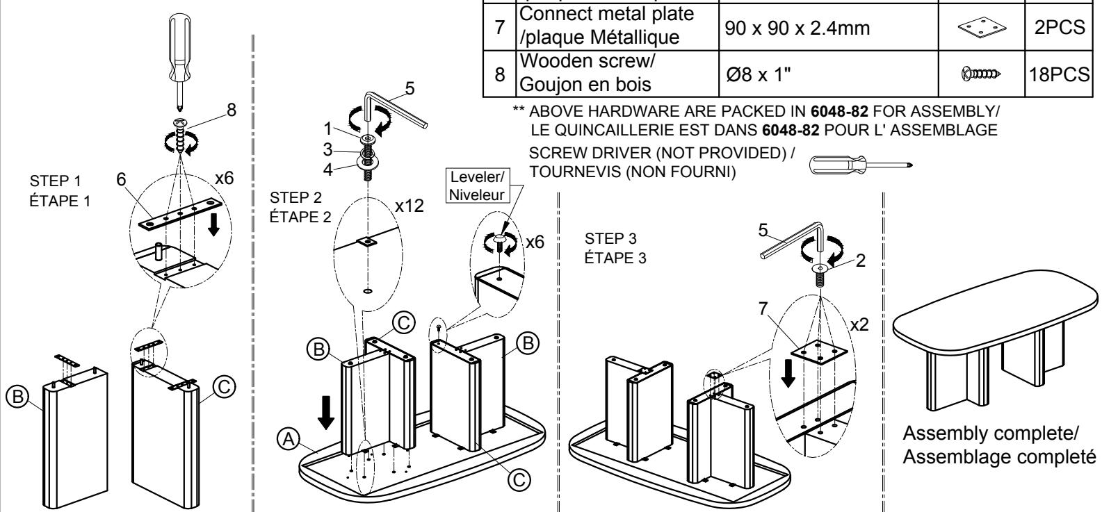
Do not tighten bolts until completely assembled
