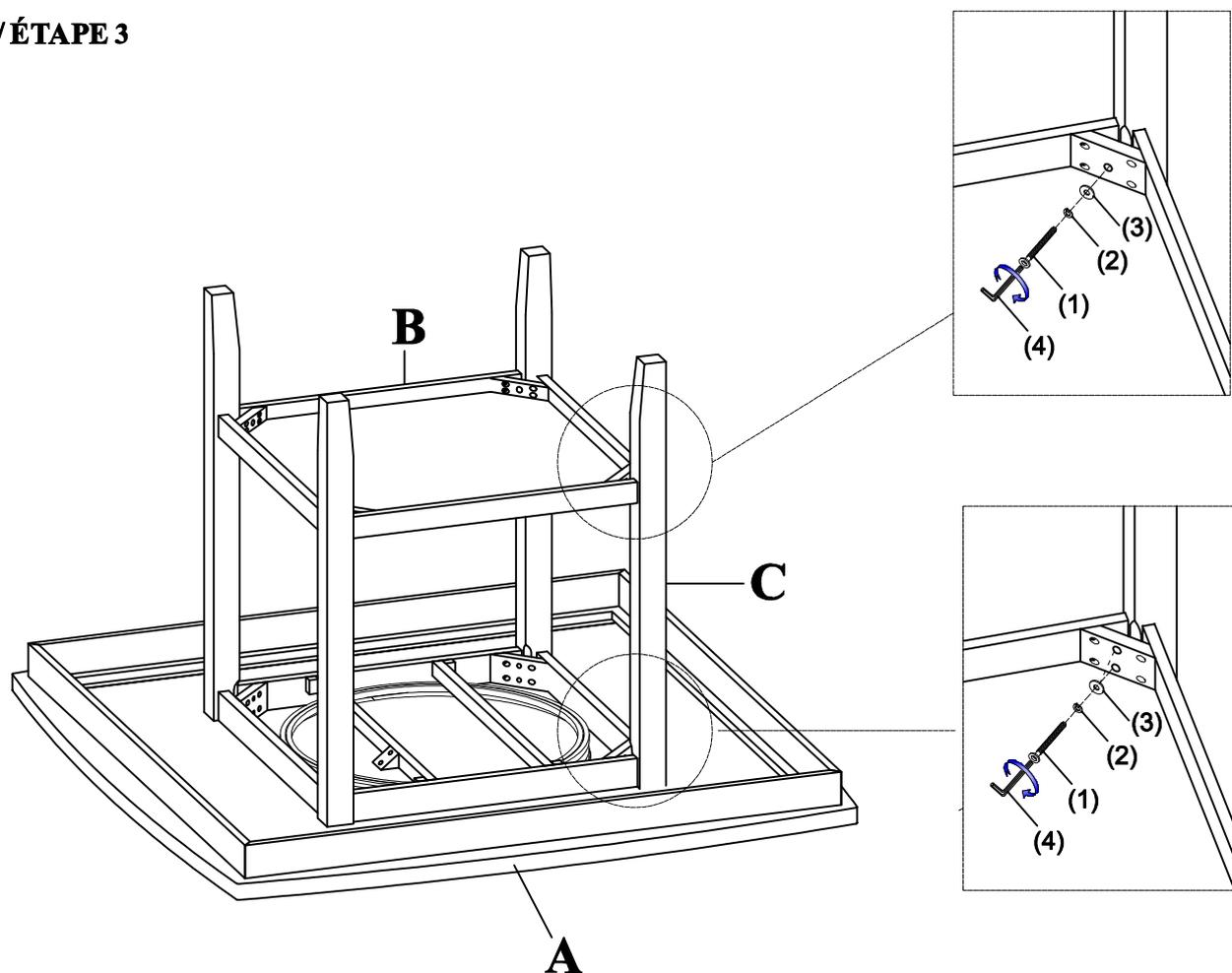
DO NOT TIGHTEN BOLTS UNTIL COMPLETELY ASSEMBLED.
