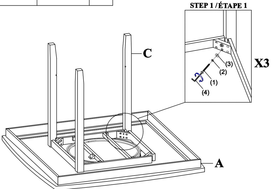
DO NOT TIGHTEN BOLTS UNTIL COMPLETELY ASSEMBLED.
