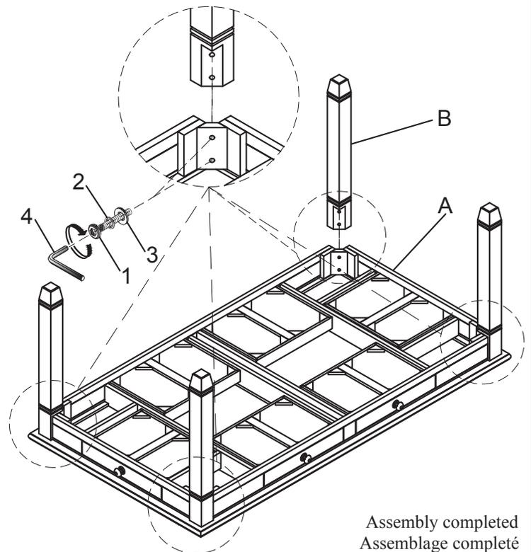
DO NOT TIGHTEN BOLTS UNTIL COMPLETELY ASSEMBLED.
