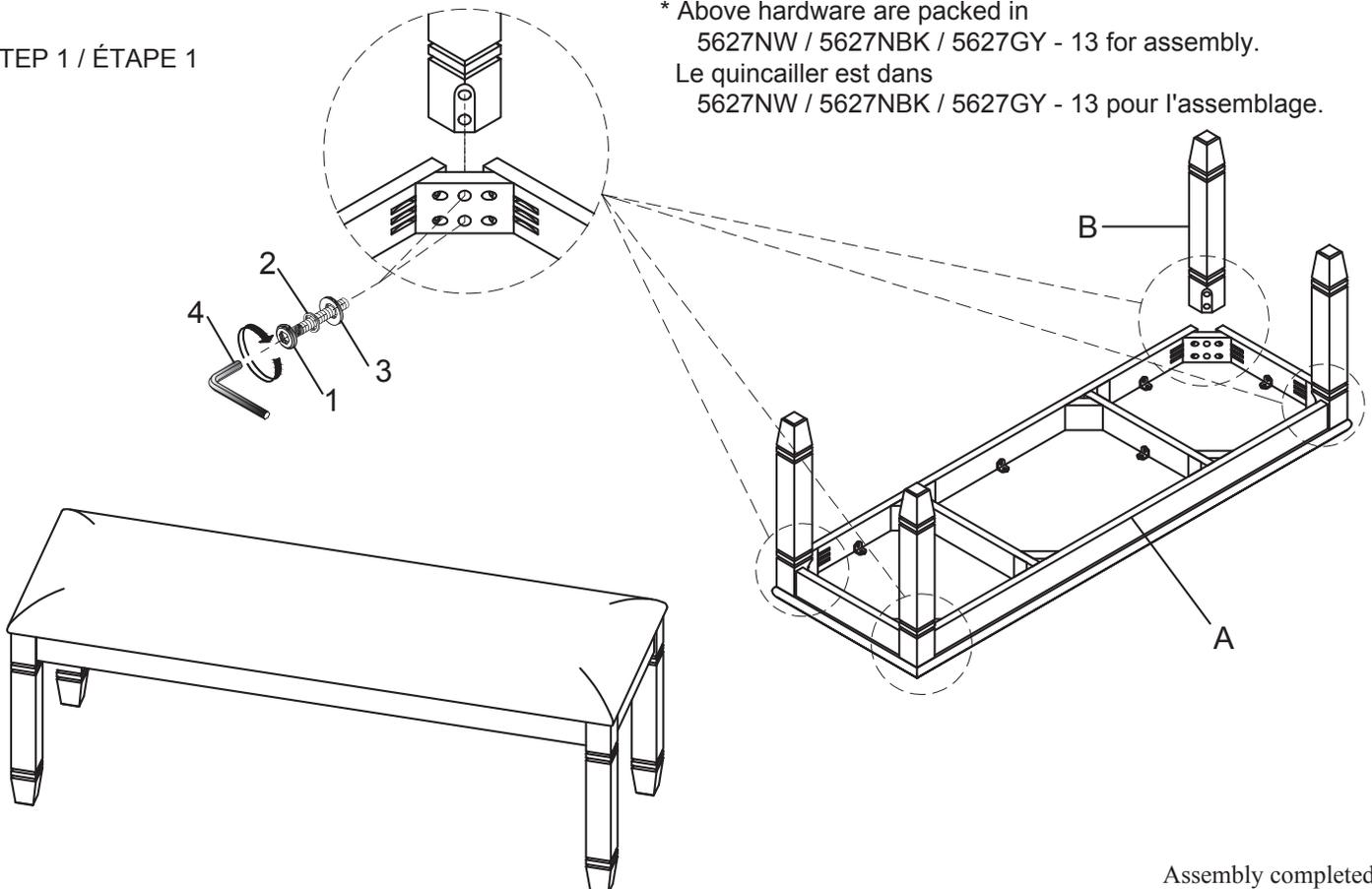
DO NOT TIGHTEN BOLTS UNTIL COMPLETELY ASSEMBLED.
