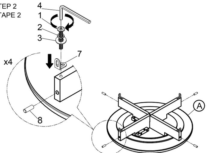
Do not tighten bolts until completely assembled
